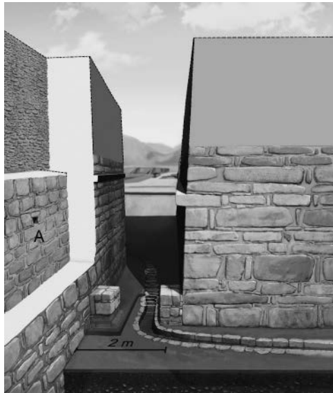
Figure 2-19 Artist's reconstruction of the passage between Building C (right) and Building D (left). "A" designates the duct in the earlier façade of Build D which leads into the Early D Gallery. ©PIACCH, drawing by Miguel Ortíz.
