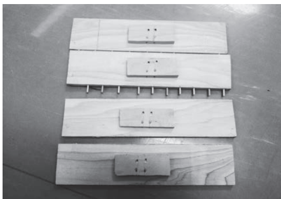
Figure 12 Wooden construction blocks like this were placed next to the exhibition of Butuan boat 2 as an interactive tool to present the construction of lashed-lug boats (Photo by Ligaya Lacsina, 2015)
