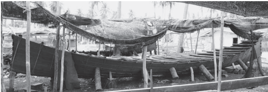
Photo 4 Timbal process of bending the board (Photo by the author on January 24, 2018)
