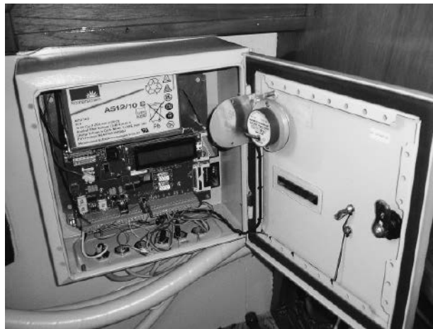
Photo 4 Automated Electronic Monitoring Box (Blue Box) for the surveillance of minke whale hunting in Norway (Photo by E. O. Øen)
