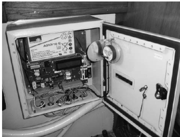
Photo 4 Automated Electronic Monitoring Box (Blue Box) for the surveillance of minke whale hunting in Norway (Photo by E. O. Øen)
