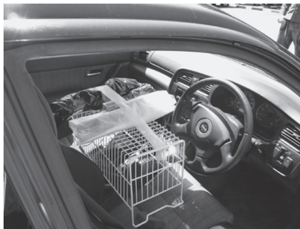
Photo 12 The high temperature treatment experiment inside a car (2010, Hidaka)
