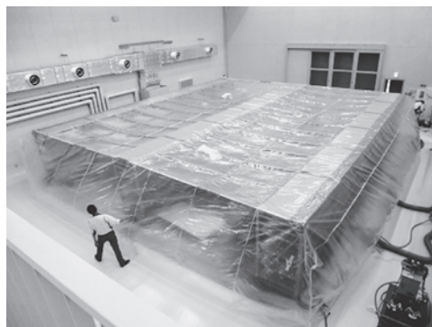
Photo 6 Large-scale carbon dioxide treatment of large wooden ships (2014, Hidaka)
