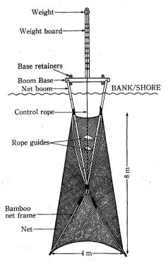
Figure 11. Plan View of a Lever Net
