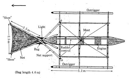
Figure 10. Plan View of a Boat-Operated Push Net
