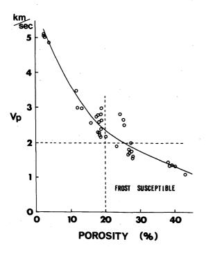
Fig. 2. The relationship between ultra-sonic propagation velocity  $(V_p)$  and porosity.
