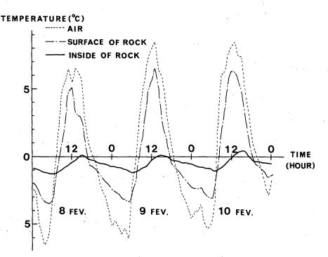
Fig. 8. Temperature changes of a rock specimen in the open-air.
