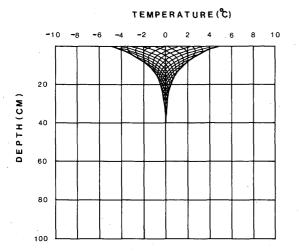
Fig. 7. Temperature fluctuation in bedrock of wet tuff (surface temperature range of +5 to  $-5^{\circ}$ C).
