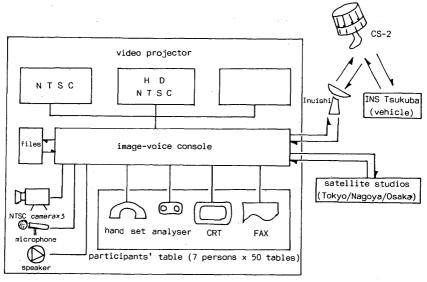
Fig 2. Conceptual Chart of INS Hall's Communication System
