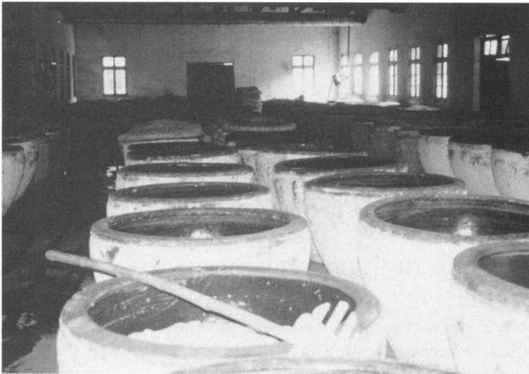
Photo 2. Earthenware pots used to prepare moromi (mash) - for shaotingjiu To produce moromi , a cup-shaped earthenware pot holding about 500 liters is used. Manufacturers can meet increasing demand by using more pots.
