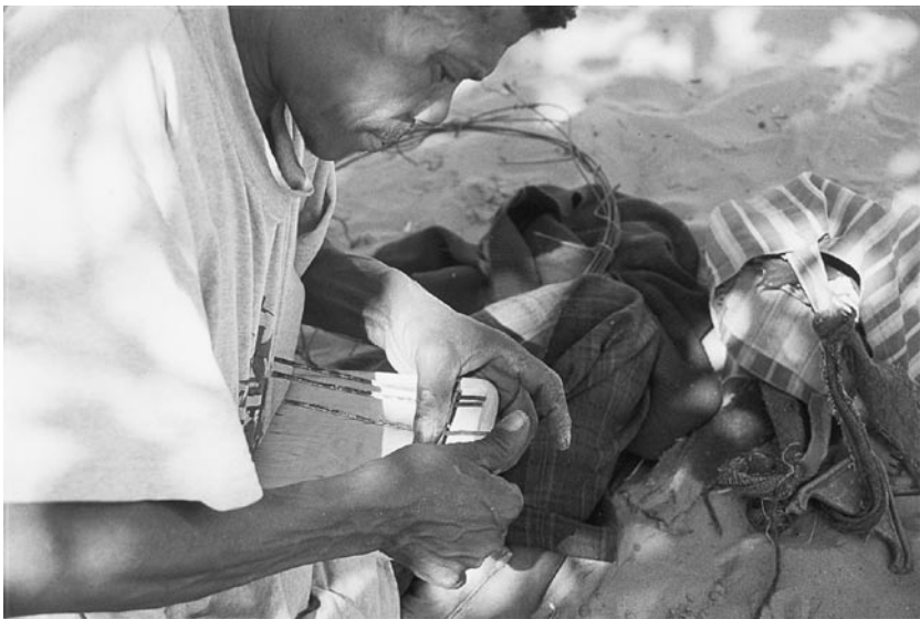
Photo 4 The keys are tuned by adjusting their lengths.
