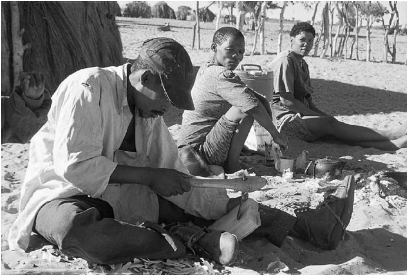
Photo 3 The thumb piano body is made by planing a roughly cut block of wood.
