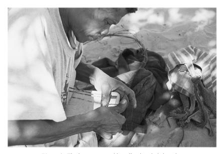
**Photo 4** The keys are tuned by adjusting their lengths.
