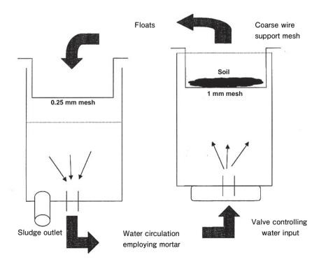
**Figure 26** The Flotation Machine Used in This Research.
