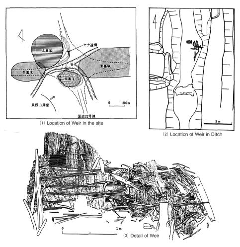
**Figure 5** Weir constructed in the trench surrounding the Asahi site (modified from Tanaka 1988).
