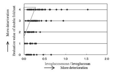
Fig. 7 Relationship between the results of the double-fold test and relative intensity of levoglucosenone in the observed pyrograms for about 140 selected volumes of the British Parliamentary Papers. The points within the triangle indicate samples that showed low mechanical strength and low levoglucosenone intensity
