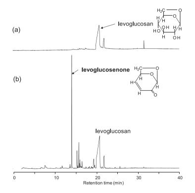
Fig. 3 Pyrograms of paper samples at 300°C: (a) an undeteriorated reference sample; (b) a highly deteriorated sample (1 cm from the edge of a page in *Censo de Poblacion*, 1932, Mexico) (Ohtani et al. 2009)
