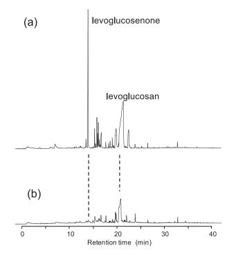
Fig. 6 Pyrograms of paper samples from identical books stored under different conditions as shown in Fig. 2: (a) open shelf and (b) stored and wrapped. The books were sampled at equivalent positions of the same page (Ohtani el al. 2009)
