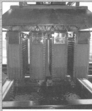
Removal of Support Paper in Enzyme Bath
