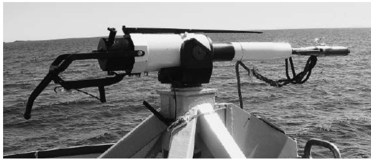
Photo 2 50mm whaling gun loaded with harpoon and Whale Grenade-99 (Photo by Björgvin Guðmundsson)
