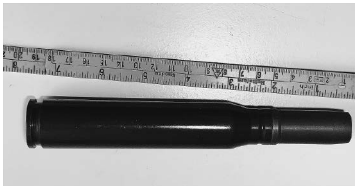
Photo 7 20mm, 15g high-velocity bullet used in hunting trials of minke whale (Photo by E. O. Øen)
