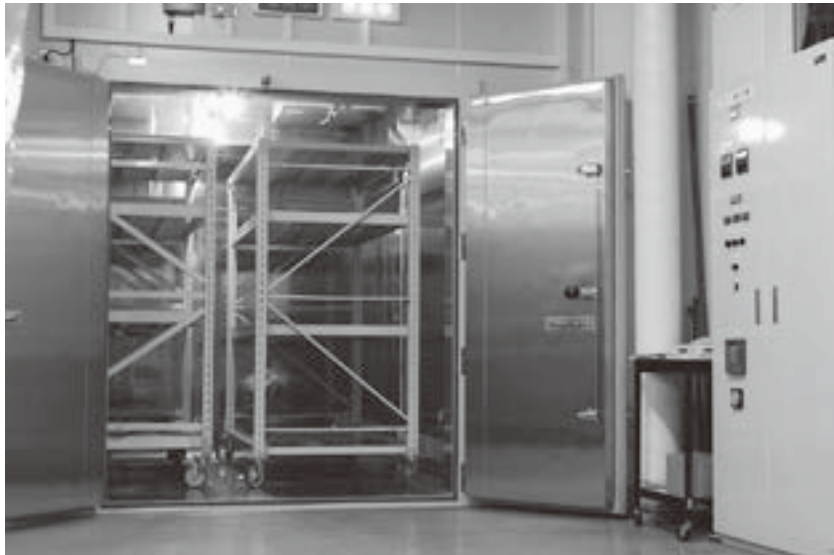
Photo 8 Walk-in heating/freezing chamber (Image by the author, July 13, 2007)
