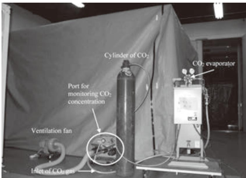
**Photo 3** The carbon dioxide treatment system: Tent size (W4000mm×D4000mm×H2500mm)
