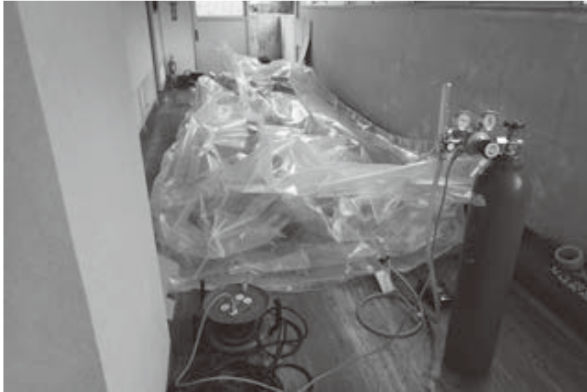
Photo 2 Objects to be treated gathered in a gas barrier plastic sheet (Image by the author, August 18, 2017)
