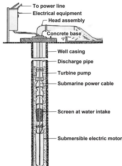
**Figure 1** Structure of a tube-well with a submersible pump
