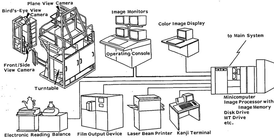
Figure 3. Image Input and Automatic Measuring System for Artifacts
