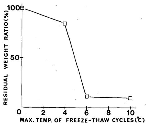
Fig. 6. Dependence of residual weight on thawing temperature.
