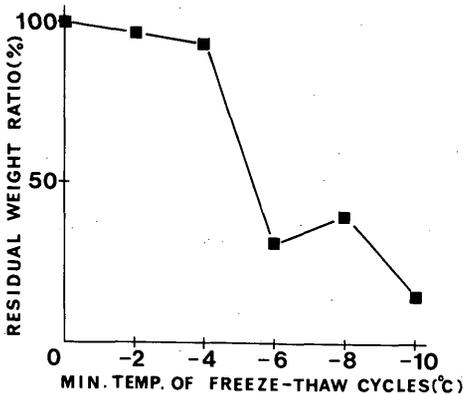
Fig. 5. Dependence of residual weight on freezing temperature.
