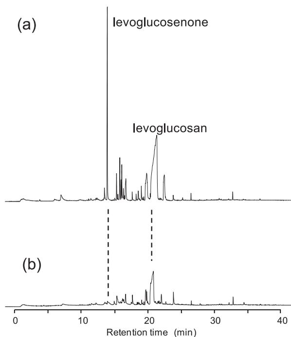
**Fig. 6** Pyrograms of paper samples from identical books stored under different conditions as shown in Fig. 2: (a) open shelf and (b) stored and wrapped. The books were sampled at equivalent positions of the same page (Ohtani et al. 2009)
