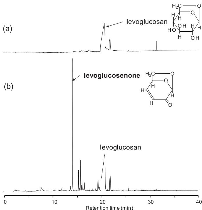
**Fig. 3** Pyrograms of paper samples at 300°C: (a) an undeteriorated reference sample; (b) a highly deteriorated sample (1 cm from the edge of a page in *Censo de Poblacion*, 1932, Mexico) (Ohtani et al. 2009)
