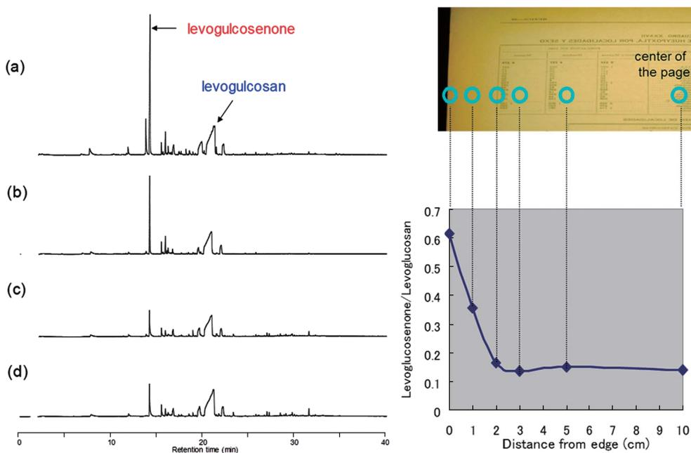
**Fig. 5** Pyrograms of deteriorated paper sampled at various positions in a page of an old book (*Censo de Poblacion*, 1932, Mexico): (a) edge; (b) 1 cm from the edge; (c) 2 cm from the edge; and (d) 10 cm from the edge (center), with the relationship between the relative peak intensity of levoglucosenone and sampling distance from the edge is also shown
