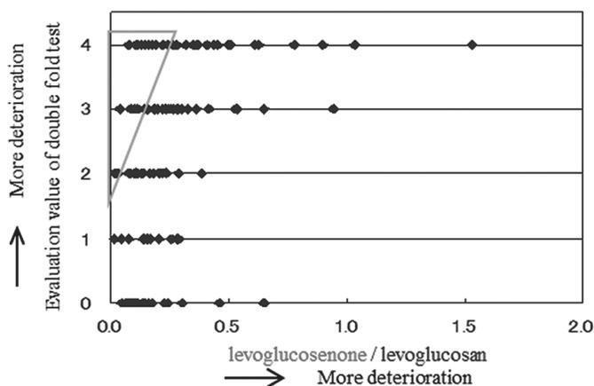
**Fig. 7** Relationship between the results of the double-fold test and relative intensity of levoglucosenone in the observed pyrograms for about 140 selected volumes of the British Parliamentary Papers. The points within the triangle indicate samples that showed low mechanical strength and low levoglucosenone intensity
